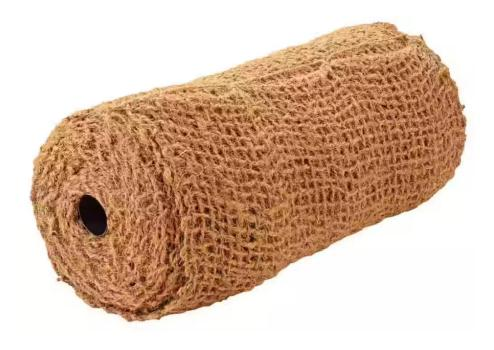
Geo-textiles are made of pure coir, drawn from the husk of the coconut, and without adding any synthetic material. It is used as a blanket to prevent soil erosion, and accelerates the growth of vegetation on banks and slopes.
