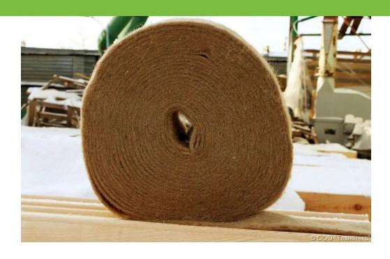
Erosion Control Blankets/Coco Mats are made using 100% coconut film. Biodegradable soil erosion control blankets are one of the most natural ways to stabilize and reinforce soil in your area. As the mat stabilizes the soil area, vegetation and other materials are able to take root.
